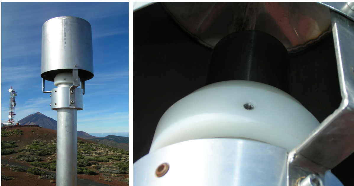
Fig. 3: Whole air inlet and sliding inner tube
