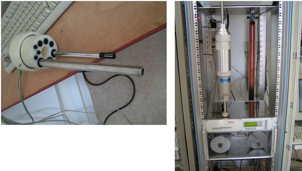
Fig 4: Flow splitter without tubing, MAAP with PM10 impactor
