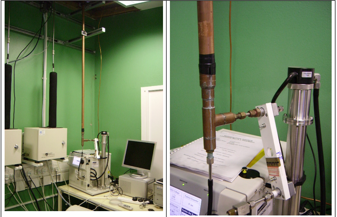
Fig. 2: Aerosol inlet at Harwell, with “virtual impactor”
