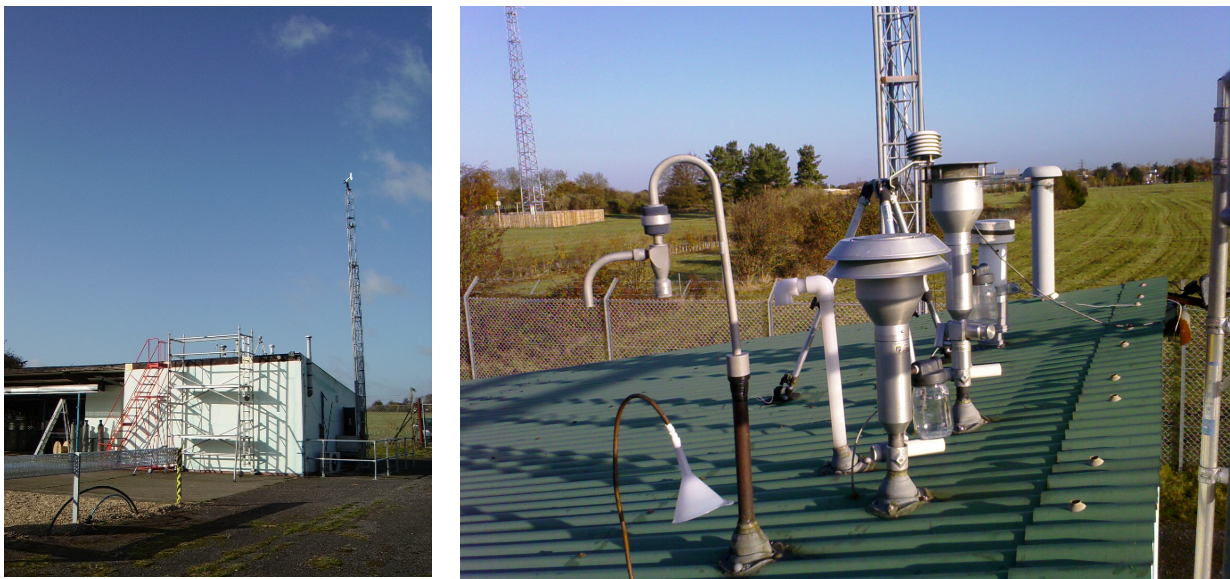
Fig. 1: Measurement site and aerosol inlets (front CPC, second SMPS with PM1 head)
