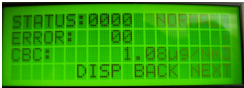
Figure 11: No indication of malfunction of the MAAP on the front panel of the instrument.
