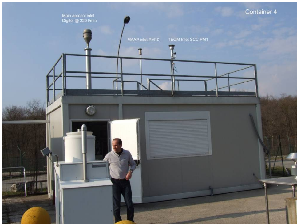
Figure 3: New aerosol container with inlets, the PM 10 TEOM is located in container 2.
