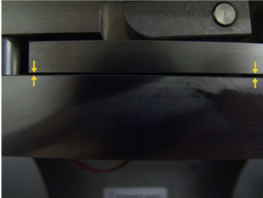
Figure 10: Filter holder of the MAAP not properly closed.
