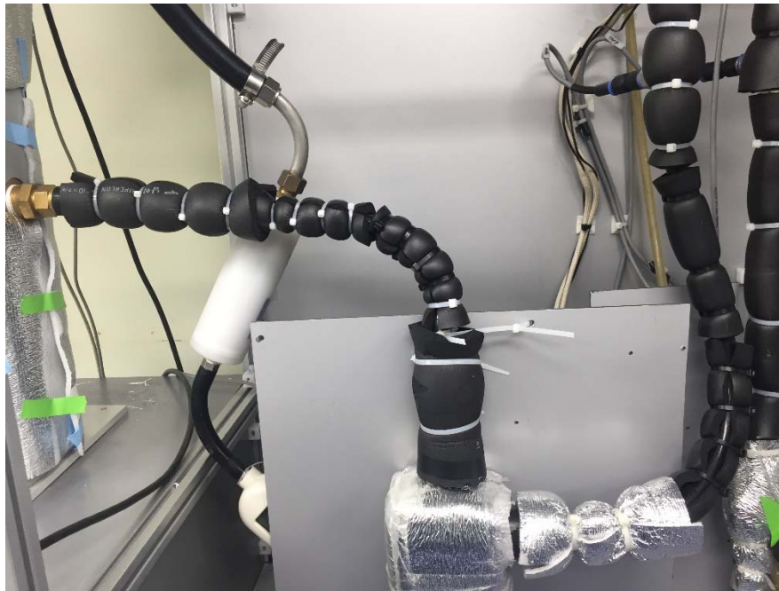
Figure 5: heating configuration of the aerosol flow tubes for the TSI integrating nephelometer (left) and the Aethalometer (right), including PM10 cyclones, respectively.
