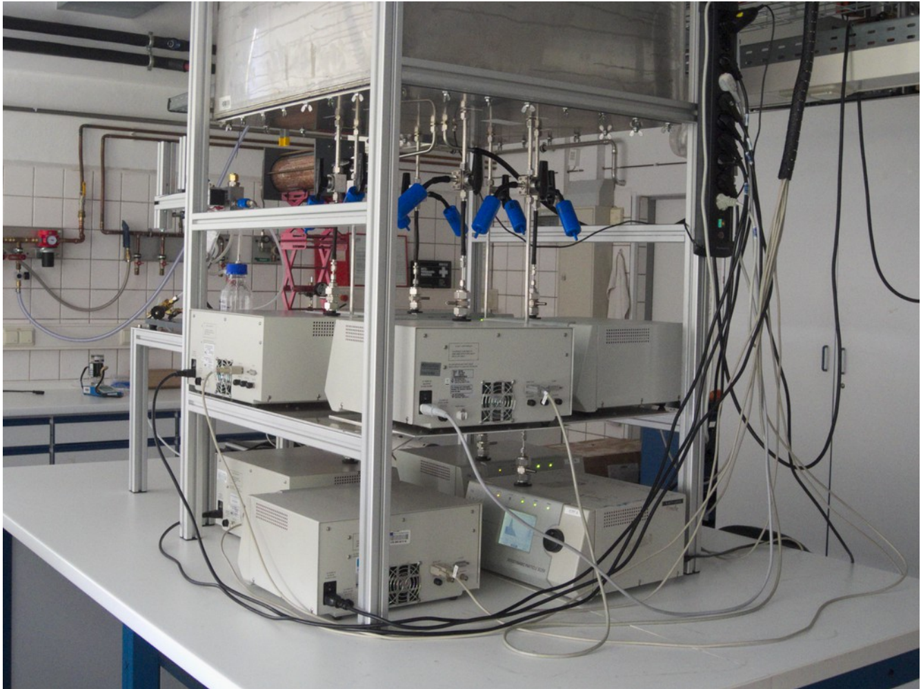
Figure 1: Measurement arrangement with mixing chamber for intercomparison of eight APS
