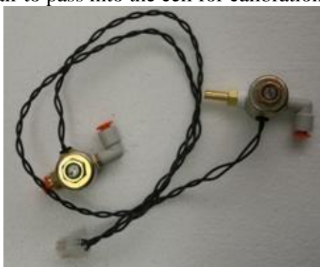
Figure 13 Span and Zero valve
