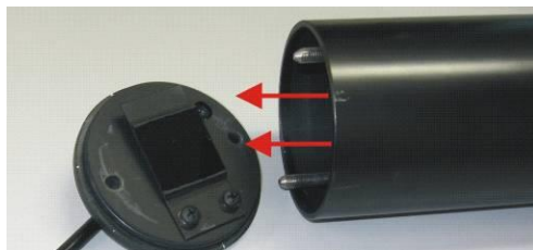
Figure 49 Removing Light Trap
