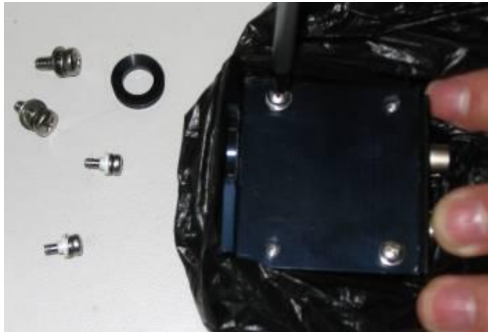
Figure 45 Removing the PMT
