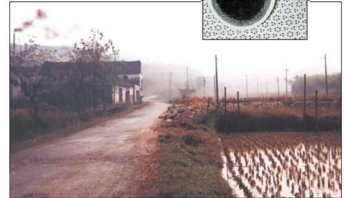
A typical hazy day near Lin An, China. Black carbon emanates from a small brick factory. (Inset) Aerosol particles collected nearby on a 47-mm Teflon filter (~8 m 3 of air sampled). The blackness of the filter indicates the presence of black carbon.
