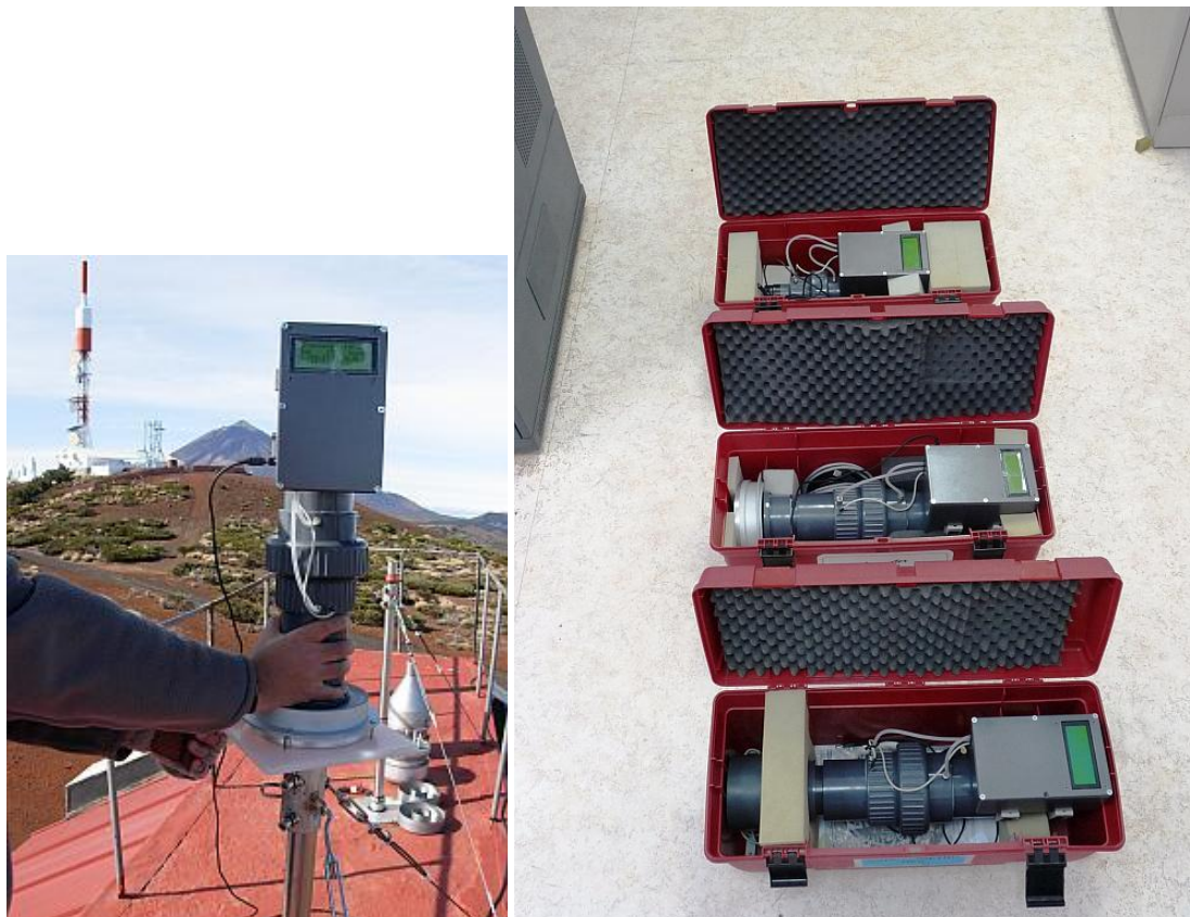
Figure 5. External flow-meter connected to the inlet of PM 10 sampler. December 2008.
